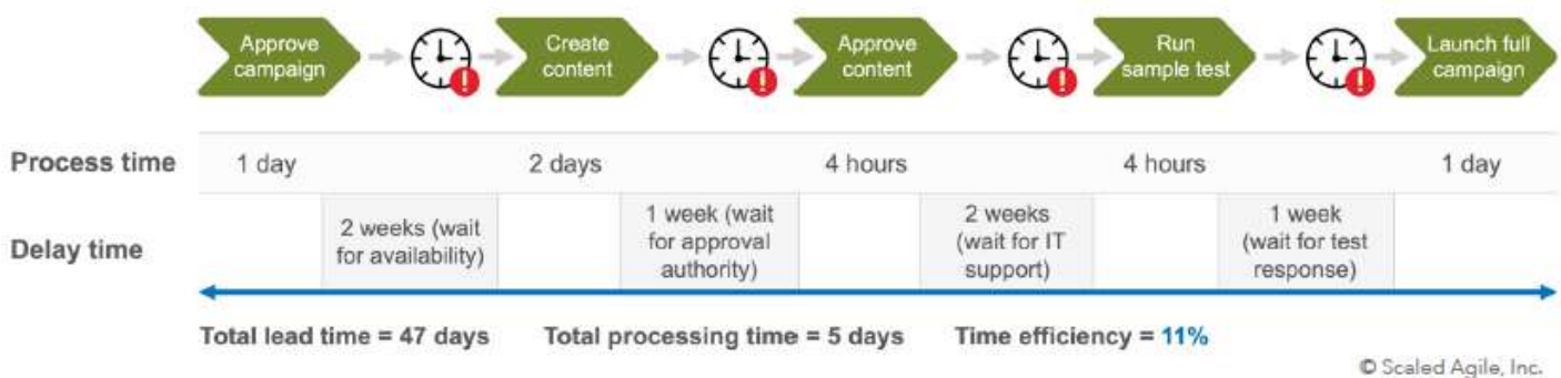
Figure 16. Value stream mapping showing processing time, total lead time, and time efficiency of a process
